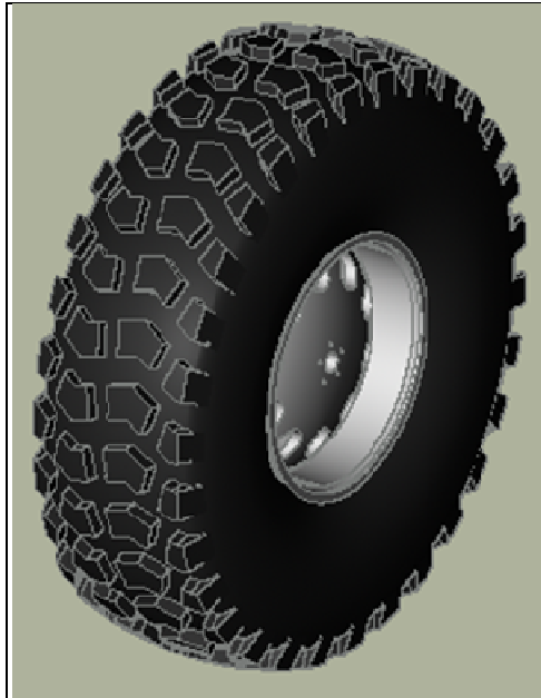
Figure 9. External view of a 395/85R20 tire with off-road tread and deepened tread grip.
