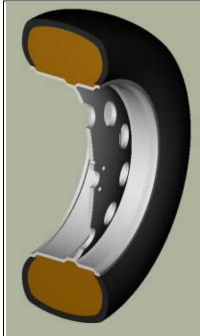
Figure 14. Visualization of air region inside a tire.
