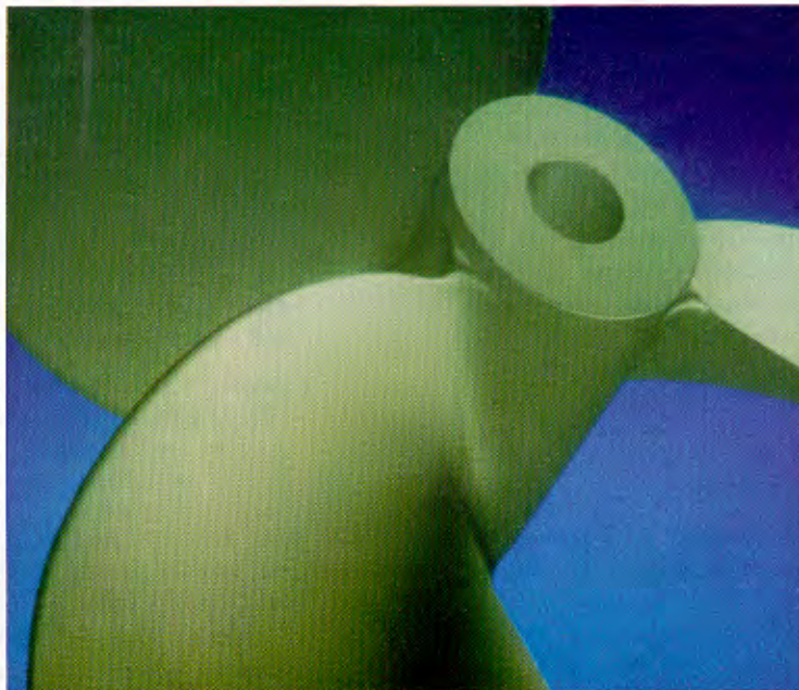
Figure 2. A geometric description of a ship screw built using spline geometry supported by the U. of Utah system, Alpha_1 . Such spline geometry can be merged into the BRL-CAD data base. The use of splines to model complex surfaces avoids the use of faceted approximations. For certain applications where high surface fidelity is required, this capability is critical. (Geometry courtesy of the U. of Utah.)
