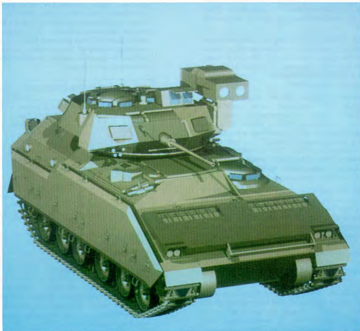
Figure 5. Frontal view of the Bradley Armored Fighting Vehicle using the BRL lgt lighting model. The geometry, built with MGED and only the primitive shapes illustrated in Fig. 1, is highly detailed so as to support high-frequency radar simulations. ( Geometric model by K. Applin, BRL. )
