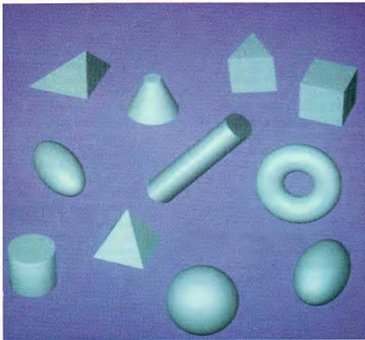
Figure 1. The set of primitive objects originally supported by the BRL-CAD environment. Basic shapes include the ARBs (four- to eight-sided planar shapes), the ellipsoid, a general cylinder, a general conic section, a torus and a (constrained) faceted object called the arbitrary surface (ARS).
