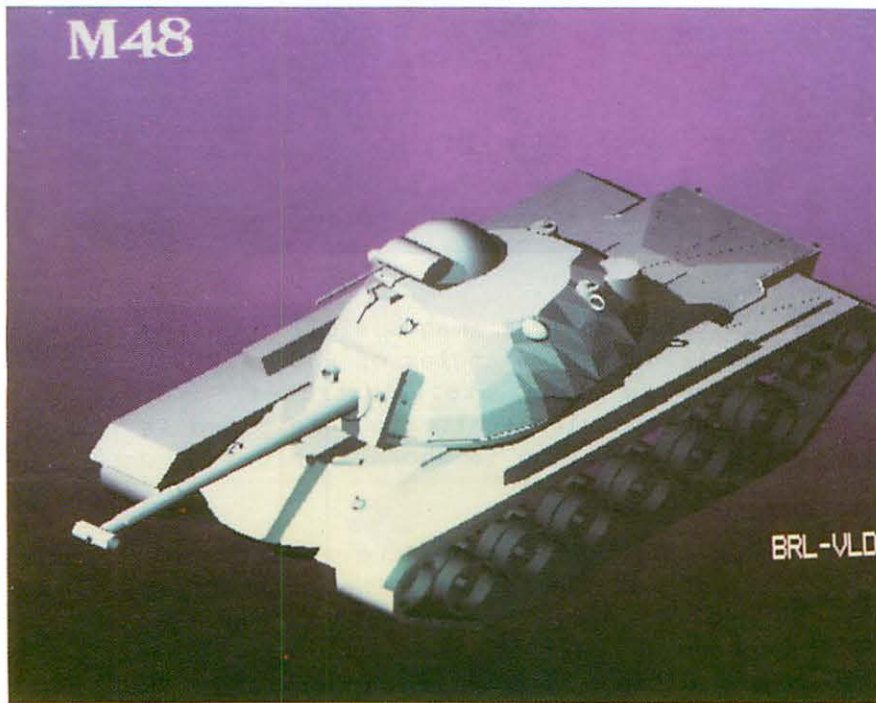
Figure 10. Color-shaded image of an M48 tank. A bistatic lighting model is used (illumination and viewing aspect angles are different) to compute the shadows. Surface reflection properties can be simulated by controlling the relative amounts of specular and diffuse contributions.
