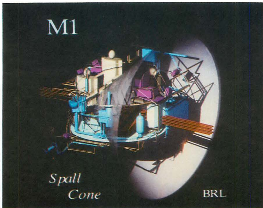
Figure 1. A portion of the interior detail of the current M1A1 target description in the region of the turret basket. The nine rods on a regular grid represent possible shaped-charge jet paths through the components. The transparent spall cone shows the domain within which behind-armor debris is likely to be generated for the hit point in question. See Reference 24 for details on how this geometry is being analyzed.
