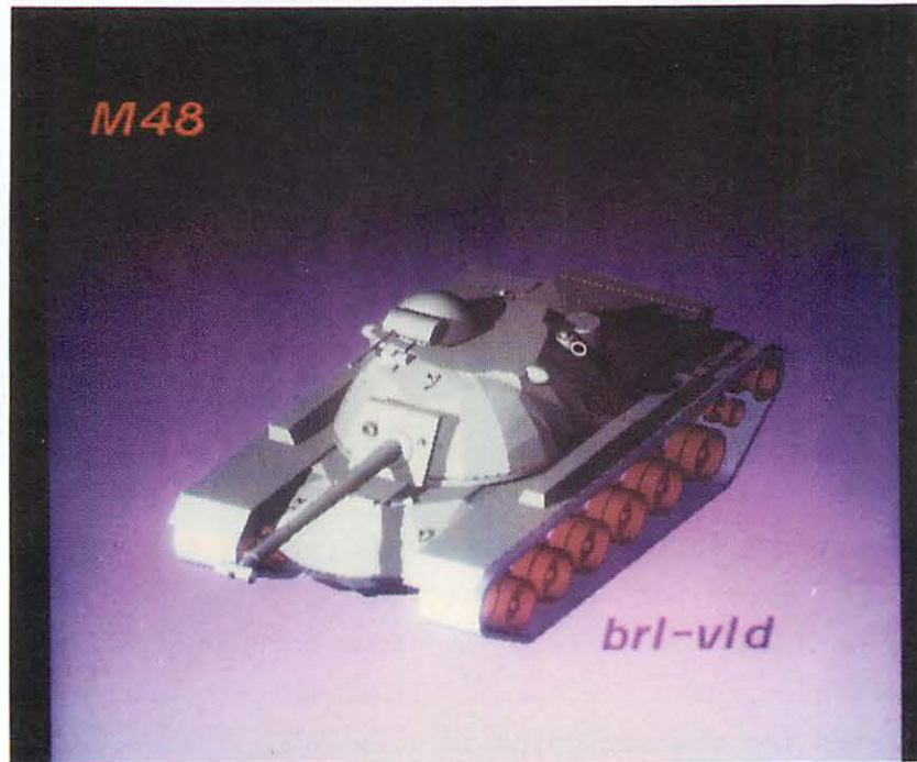
Figure 2. An image of an M48 tank as it has been described for many years. Compound surfaces, such as the glacis and turret, have been approximated using a series of triangular facets.
