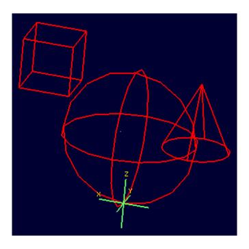
BOTH the object1.c present in bigobject.r and the definition of object1.c in object3.c have been translated - only one instance of the sphere and cube combination is visible. This is a subtle problem, but remember the original goal was to move ONLY the object1.c inside bigobject.r - this technique moved more than that. It would be especially problematic if a modeler didn't realize that object1.c was still in the display
