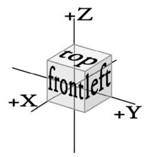
The preceding diagram was created to illustrate BRL-CAD's coordinate system.
