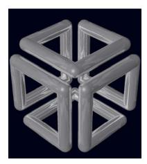
BRL-CAD can run series of commands piped in or redirected to it via standard input, and it is considerably more efficient to batch multiple BRL-CAD commands together via standard input instead of re-invoking BRL-CAD for each command. The image demonstrates the output of a shell script that uses BRL-CAD tools to procedurally create and render the SGI Cube. For more information, go to <a href="http://brlcad.org/wiki/SGI\_Cube">http://brlcad.org/wiki/SGI\_Cube</a>.
