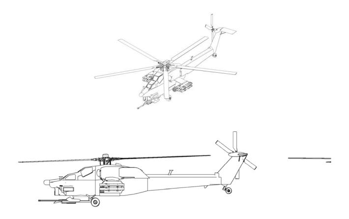
This raytrace image is a multiple-view hidden line rendering of an Mi28 Havoc Russian attack helicopter using BRL-CAD's rtedge utility. The model is entirely composed of implicit primitives combined together with CSG boolean operations.
