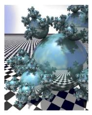
BRL-CAD provides a comprehensive procedural geometry interface as a means for creating models algorithmically instead of manually. This screenshot shows a classic "Sphere Flake" model with five levels of recursion, specular reflections, multiple light sources, environment mapping, checkered texture synthesis, ambient occlusion, and soft shadows.
