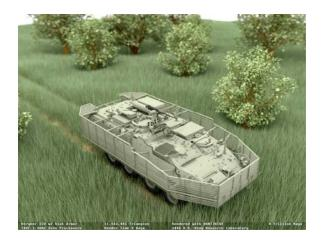
Representing more than 8 trillion rays fired at this 11-million-polygon scene (amounting to more than 20 million rays per second on 2004 hardware), this figure signifies the path tracing capability of BRL-CAD. A full light simulation was computed to generate the image with all exterior and interior vehicle detail, including every nut, bolt, wire, and component inside the vehicle and every leaf and blade of grass modeled as actual geometry (with no textures and no procedural geometry).
