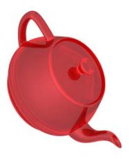
Boundary representation NURBS surface geometry is one of the dominant geometric representation formats in CAD. BRL-CAD is one of the few 3D solid modeling systems that not only support geometry in boundary representation NURBS format but also provide extensive support for robust solid ray tracing of NURBS geometry. The image shown is the classic computer graphics Utah teapot model prepared for 3D printing and rendered via BRL-CAD ray tracing.
