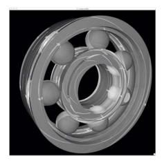
Raytracing is central to BRL-CAD as a means for performing geometric analysis (e.g., calculating weights and moments of inertia) and for rendering images for visualization purposes. The image shown is a BRL-CAD 2D framebuffer screenshot displaying the rendering of a ball bearing. The bearing is modeled with a material appearance resembling acrylic glass, and this raytracing result shows reflection, refraction, shadowing, and some caustic effects.
