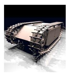
BRL-CAD focuses on solid modeling CAD. Solid modeling is distinguished from other forms of geometric modeling by an emphasis on being physically accurate, fully describing 3D space. Shown is a 3D model of a Goliath tracked mine, a German-engineered remote controlled vehicle used during World War II. This model was created by students new to BRL-CAD in the span of about 2 weeks, starting from actual measurements in a museum.
