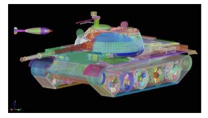
As shown, a BRL-CAD target description can be converted to a finite element mesh (FEM) using the BRL-CAD g-sat exporter and Cubit from Sandia National Laboratories.
