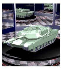
While now a fully hybrid modeling system, BRL-CAD has its roots in CSG modeling with implicit primitives. This image, provided courtesy of GSI Solutions, Inc., depicts a detailed M1A1 tank on a pedestal in a mirrored showcase room. The model is entirely constructed from implicit primitives and CSG boolean operations.
