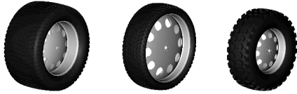
Examples of procedurally generated tires - from left to right, dimensions are 505/50R24, 315/50R50 and 325/40R32
